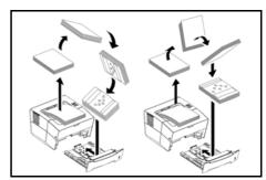
**NOTE:** Nothing will be printed on the instruction sheet. If the paper is curled, straighten it out before loading the paper in the cassette.
